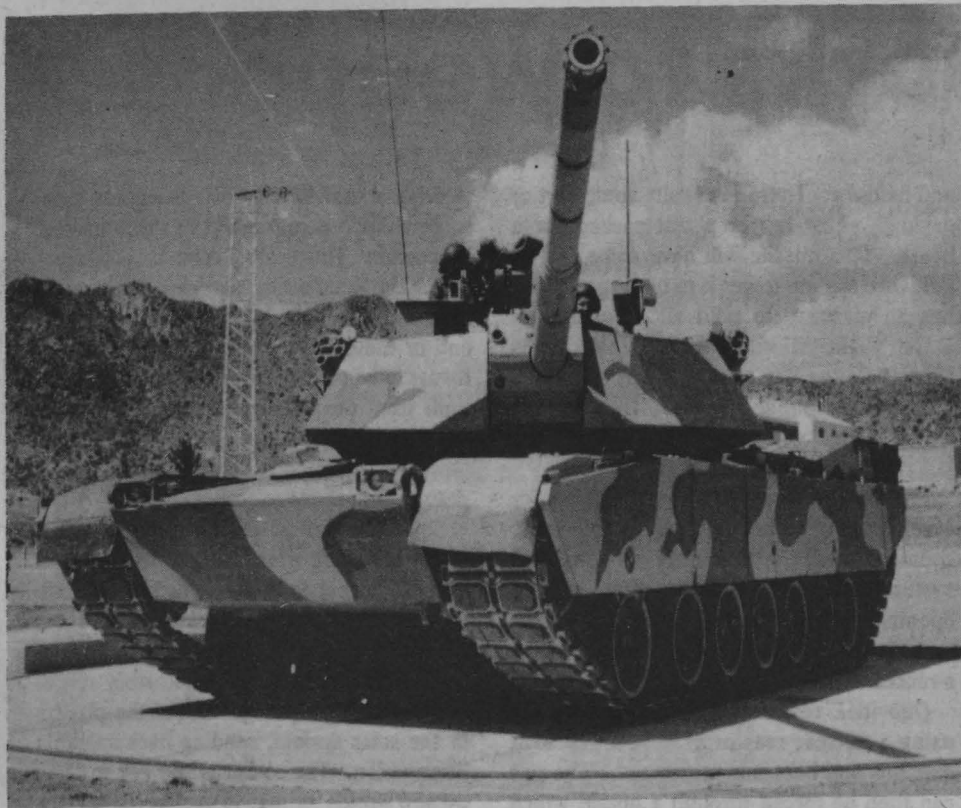
XM-1 TANK—A close up view of the XM-1 tank and the XM-250 smoke grenade launcher. This is the Army's newest piece of equipment and has under gone testing here at the range. (Photo by Frank Trevino)
