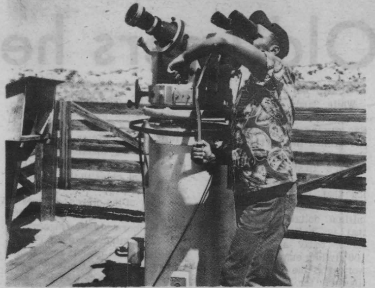
EARLY CINETHEODOLITE - Picture taken in 1949 shows pioneer Land-Air employe operating early cinetheodolite - German-made Askania surveyor's theodolite combined with a motion picture camera. Tracking was manual. Board fence around the ground-level instrument was built to keep out curious cattle. Modern cinetheodolites are housed in astrodomes and have power driven tracking systems. (Land-Air photo by B.M. Reavis)
