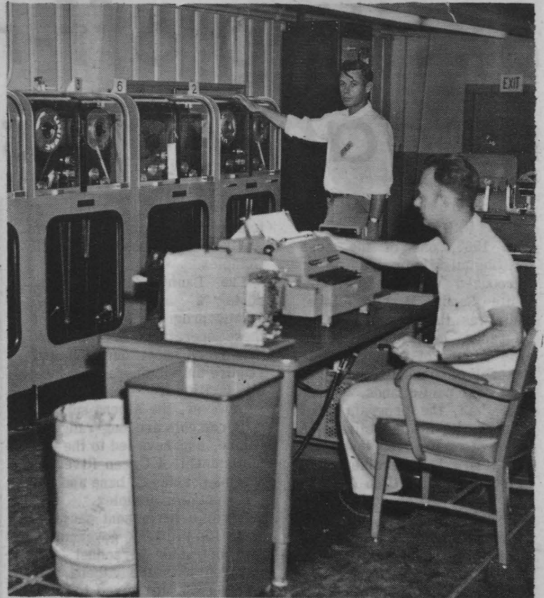
COMPUTER OPERATION - The site of the art in computer input/output devices is shown in this picture taken at Holloman Air Force Base in 1958. Dr. Garner McCrossen, left, and Billy G. Medley are operating the UNIVAC 1103-A computer. This was one of three large-scale scientific computers used at WSMR for data reduction, missile ballistics and some of the early real-time applications. (Photo courtesy UNIVAC)
