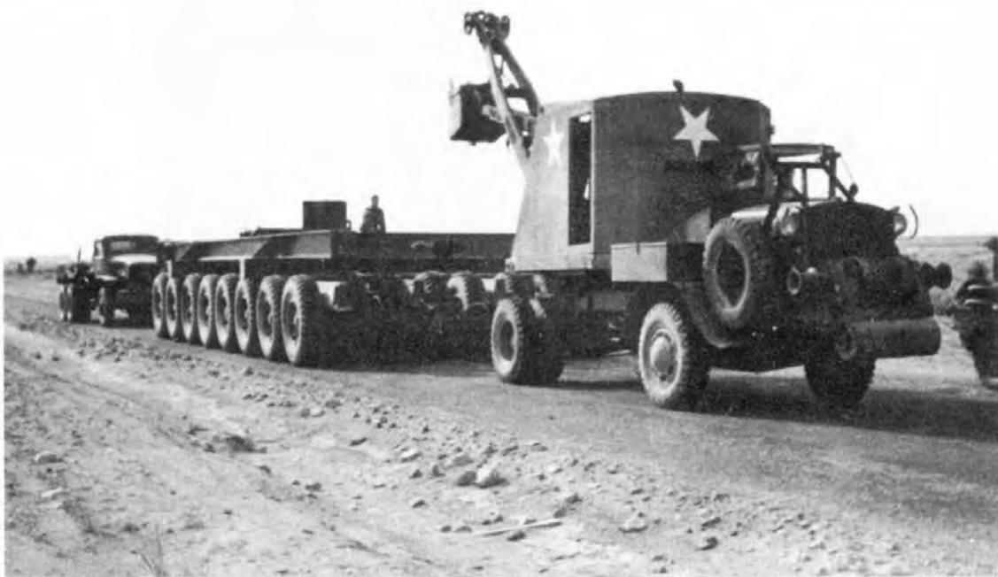
Figure 22. Scoop shovel used for hauling unloaded Jumbo carrier. The 2-ton trucks in the rear were for braking. *Courtesy Marvin Davis.*
