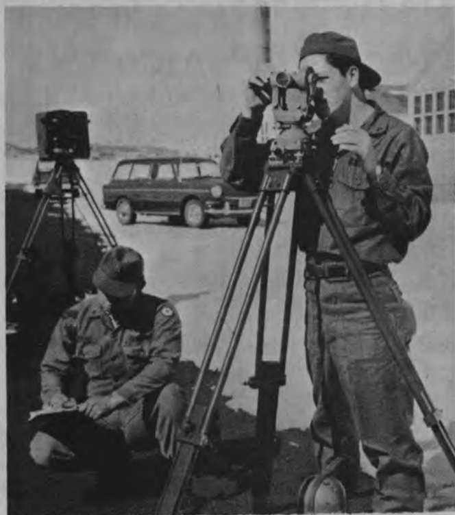
MAPPING — SP4 Raymond Markus (standing) and PVT Terry Cowan, both of the Arizona Gravity Survey (537th Engineers) map an area in northern Arizona. They are using the Wilde T2 transit survey instrument. In the background is the Teleremoter, a microwave distance measuring instrument. The equipment is serviced by the Navajo Army Depot near Flagstaff. (U.S. Army Photo)
